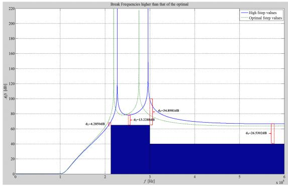
Fig. 8: Comparative plot of the optimal break frequencies in green (fstep=[2.13MHz 3MHz]) and higher break frequencies in blue (fstep=[2.2MHz 3.3MHz]).
