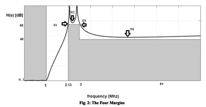
The design specification calls for the transmission zeros to be placed such that the margin between the actual and specified stopband loss is the largest possible. The design goal therefore is to make D1, D2, D3, and D4 equal, or close enough to equal so that they are all as large as possible.
