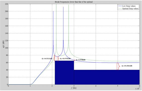
Fig. 7: Comparative plot of the optimal break frequencies in green (fstep=[2.13MHz 3MHz]) and lower break frequencies in blue (fstep=[2.0MHz 2.7MHz]).
